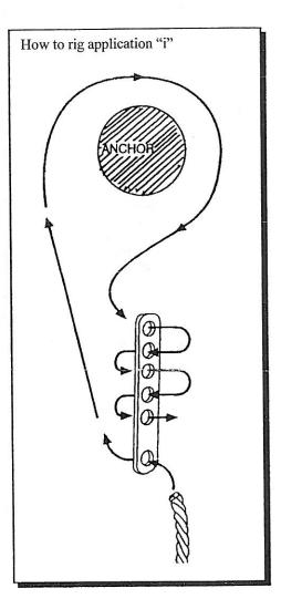
☐ Knots shall not be used for load bearing end terminations.
