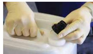
2. Remove 33 mm cap from the jug and remove foil seal. Attach 33 mm quick connect cap by tightening clockwise.
