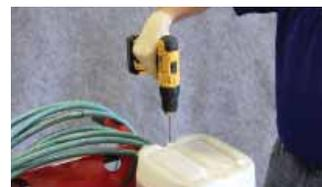
5. Remove the quick flow cap and finish drilling quick flow port with a ¼ drill bit.
