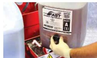
1. Locate the quick connect fitting on the side handle of each A-side and B-side 5-gallon jug. Next remove quick connect fitting from side handle.
