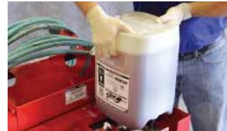
3. Using the top handle and side loading handles, invert 5-gallon jug container onto urethane dispensing cart.
