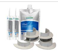
**E-Curb kits** include bisected circular pieces with inside diameters of 3, 4, 5, 6 or 9 inches, a  $4.5 \times 3.4$  inch rectangle, 1-Part Pourable Sealant and M-1 Universal Adhesive/Sealant to complete installation.
