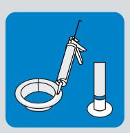
Prime penetrations using M-1® Universal Sealant/Adhesive, extending up 3 inches from the base and tool in. Apply three 1/4 inch diameter beads to the bottom of each curb section.
