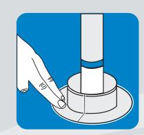
Press the curb in place. Seal around the joints and outside of the curb with a bead of M-1 and tool to ensure a monolithic seal.
