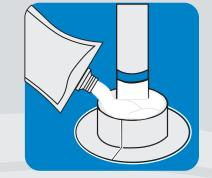
Fill curb with 1-Part® pourable sealer when installing around high movement details and on granulated surfaces.
